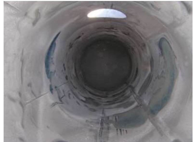
Tiger striping on worn shell
