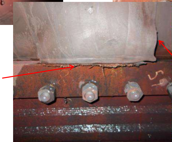
Horizontal Tear along the clamping bar
