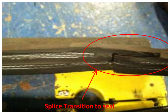
Failed Seal Splice
