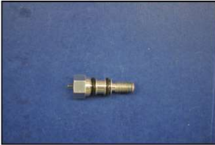
Photograph 6 Orifice Fitting Removed from Relay
