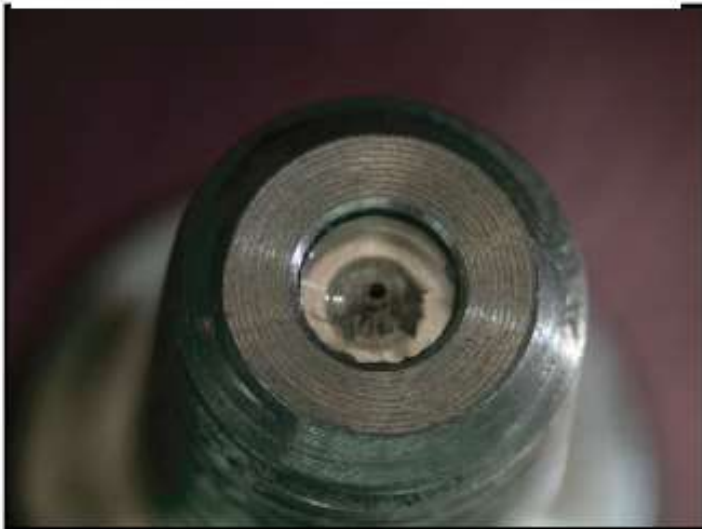
Photograph 7 Orifice Hole After the Piece of Foreign Material had been Dislodged
