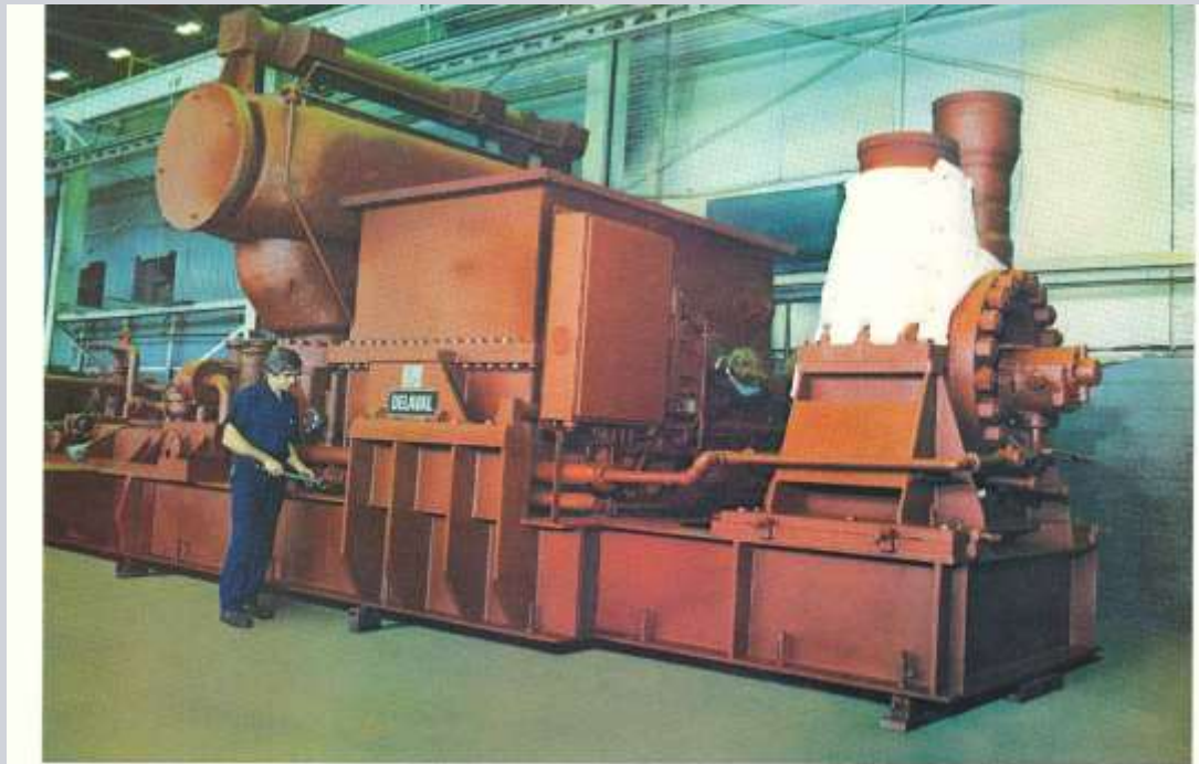
DELAVAL REACTOR FEED PUMP 16,000 HP TURBINE WITH ITS REACTOR FEEDWATER PUMP MOUNTED ON A CONTINUOUS BEDPLATE - STEAM CONDITIONS - 96 PSIA/490°F PRIMARY - 883 PSIA/550°F SECONDARY PUMP CONDITIONS - 20,000 GPM @ 2460' TDH @ 5400 RPM.
